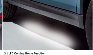
Upon opening front doors, the area below the front doors of the vehicle is illuminated to assist passengers to find their way.
