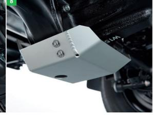
8 | Rear Differential Guard Made of 3mm aluminum plate. Part No. 9912J-78R41-000
